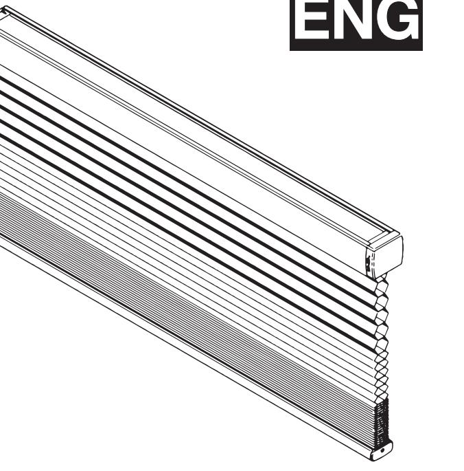
Identify the head of the motor housing on the right side of the shade (see drawing) - Press the PROGRAM button until the shade oscillates (the shade will oscillate - a quick back and forth movement of the shade) Press the UP button on the remote (see drawing) - the shade will oscillate again - the motor and transmitter are now mated.
