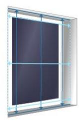
Measure the full width and height of the recess [the size inside the window frame opening] and we will make the appropriate deductions to ensure a perfect fit.
